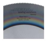
MEBA **PRO+** is a surface coating with 2,5 microns thickness layer, with a Titanium and Carbon base, which gives a high hardness and a low friction.
