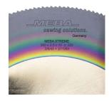
MEBA **XTREME** is a surface coating with 3 microns thickness layer, with a Titanium and Aluminium base, combining high toughness of the multilayer structure with high hardness. It allows machining at high speed, with few lubricant.
